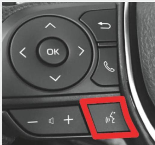
Push and hold the voice command talk switch for 2-3 seconds to activate Siri
